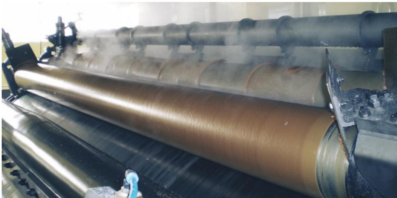
Starch drying on a drum dryer
