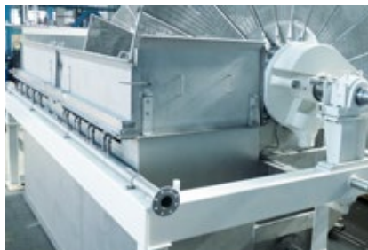
STARDISC: The common trough is applied with an agitator, making the filter suitable for products with highest solids densities.
