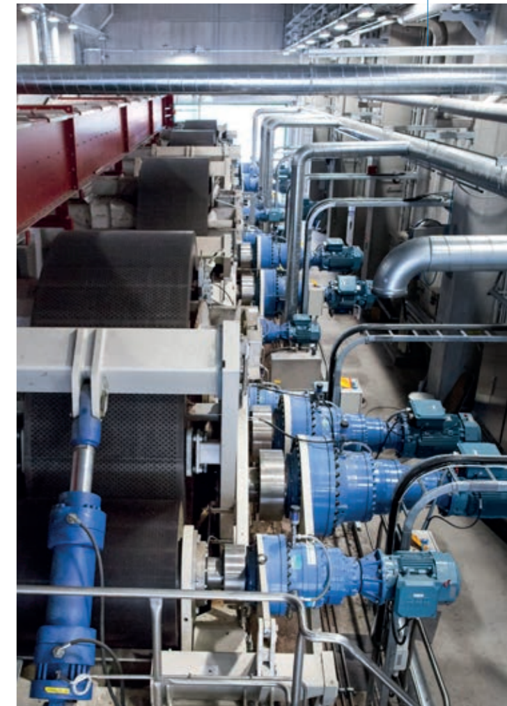
One of the new, key technologies introduced to the woodyard is the new generation bark press, ANDRITZ HQ-Press, which targets to deliver around 5%-unit higher dry solids content of bark than any other press on the market.
