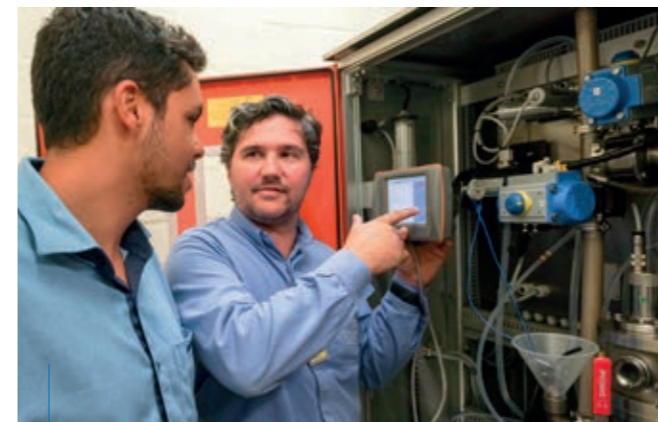
Daniel Scigo of Eldorado, demonstrates a new smart sensor (an online shive measurement device) that is a new input to the APC strategy for Eldorado's fiberline. This ability to easily add new variables into existing controls is part of the OPP software strategy leading to an Autonomous Mill.
