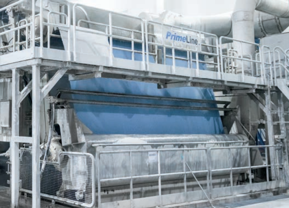
The two tissue machines are currently unique on the Asian market because they combine a high-performance Yankee with a steam-heated hood.
