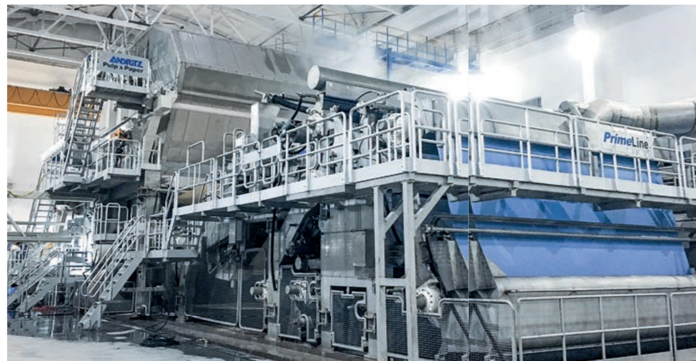
ANDRITZ supplied two identical tissue machines, PrimeLineSTs , with design speeds of 2,000 m/min and a width of 5.6 m each.
