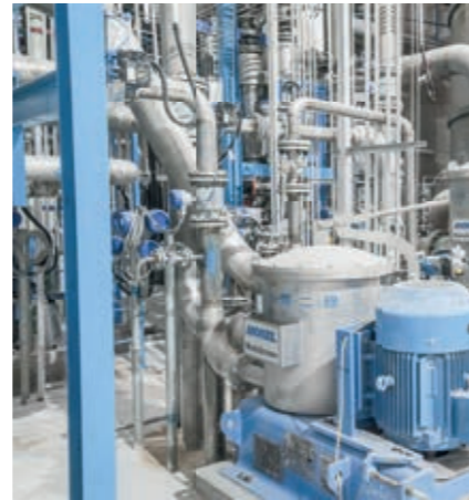
The stock preparation system consists of two lines. One is for LBKP market bale, and the other one for bamboo self-made slurry pulp.
