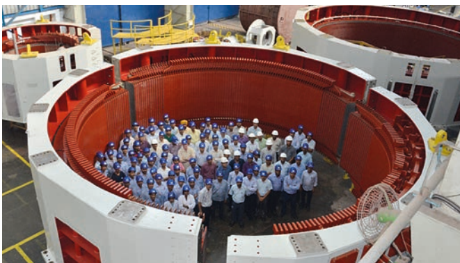
Manufacturing of stator for HPP Xekaman 1
