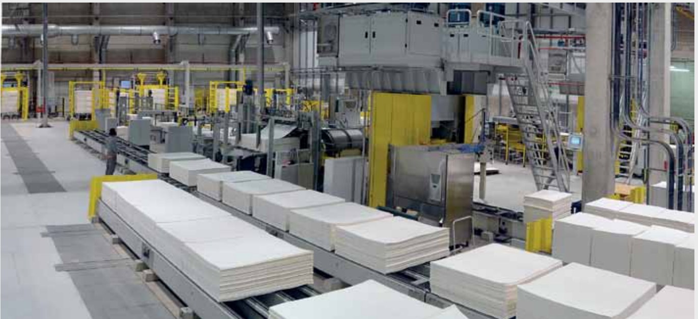
▲ Automated baling lines in operation, each achieving peak productions above 300 bales per hour.
