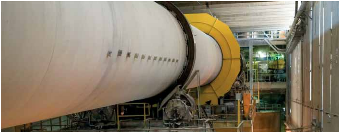
▲ The Skowhegan kiln is inside a building. The switch to natural gas replaces the equivalent of 80,000-100,000 barrels of No. 6 fuel oil each year in the kiln.
