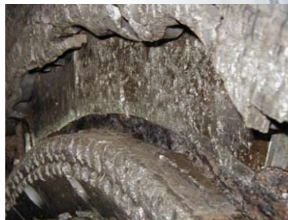
New refiner disc plate (above) and heavily damaged refiner disc (below) after a plate clash.
