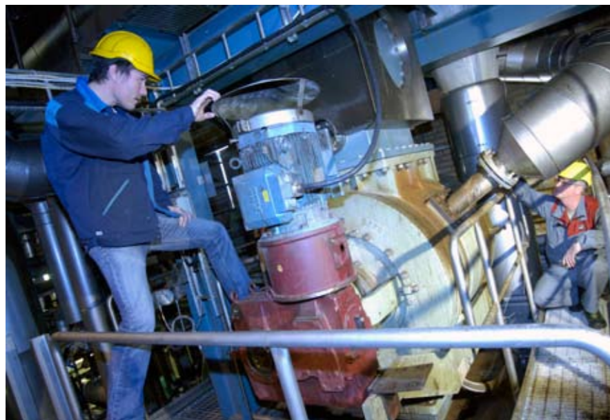
Ulf Lundström, Customer Service Manager for Andritz's Pulp Mill Services Division in Sweden, checks the chip feeding mechanism on Cooking Line 4.
